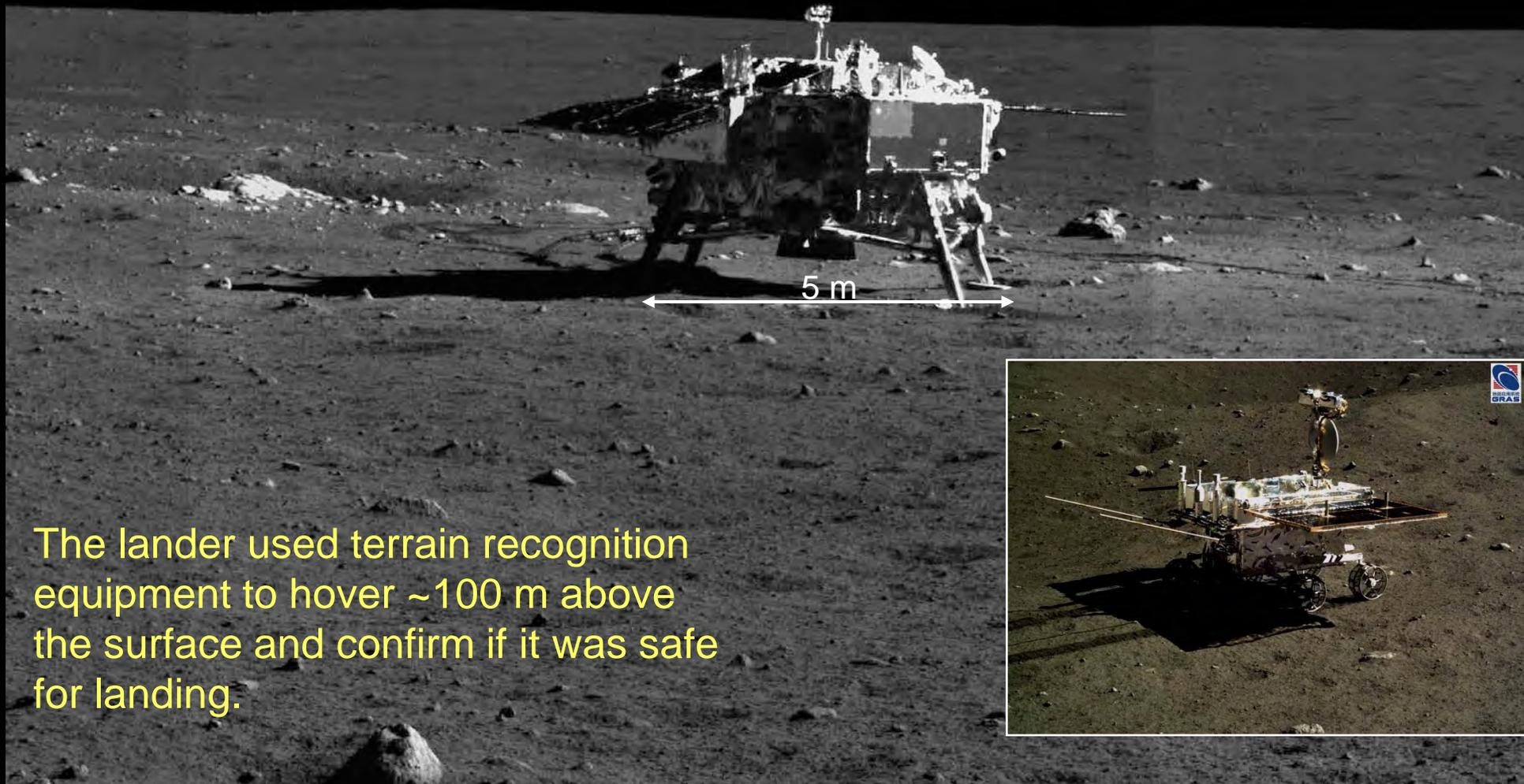
The lander used terrain recognition equipment to hover ~100 m above the surface and confirm if it was safe for landing.
